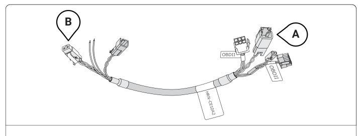
**Step 4** : Remove and insert the EOL resistor into the gray Y connector on the HRN-CE10A2 harness (labeled **A** in the image).
