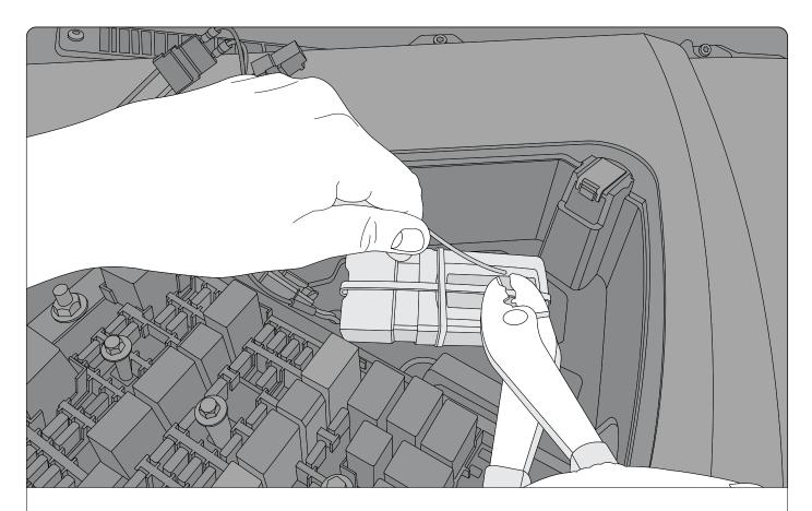
Step 7: Use zip-ties to secure the GO device and harnesses.
