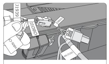
Step 6B: Connect the OBD II-labelled 6-pin black Molex connector from the HRN-CK10A2 harness to the OBD II-labelled 6-pin black Molex connector from the HRN-CM24Y1 harness.
