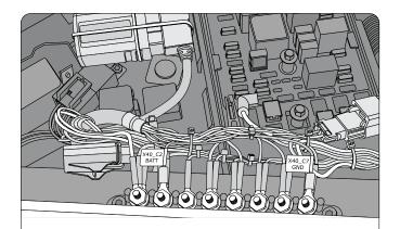
**Step 7:** Plug in the GO device, and use zip ties to secure the device and harnesses.
