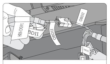
Step 6A : Connect the OBD II-labelled 12-pin black Molex connector from the HRN-CK10A2 harness to the OBD II-labelled 12-pin black Molex connector from the HRN-CM24Y1 harness.
